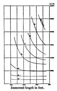
Fig. 42.—Curves of E.H.P. for 1,000-ton Ship. Group "A." Type 3. Block Coefficient .516.
