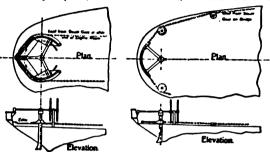
FIG. 123.-Steering Gear of Merchant Ship.
