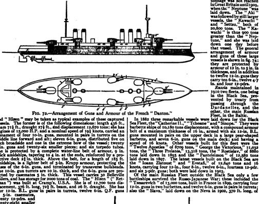
Fig. 72.-Arrangement of Guns and Armour of the French "Danton."
