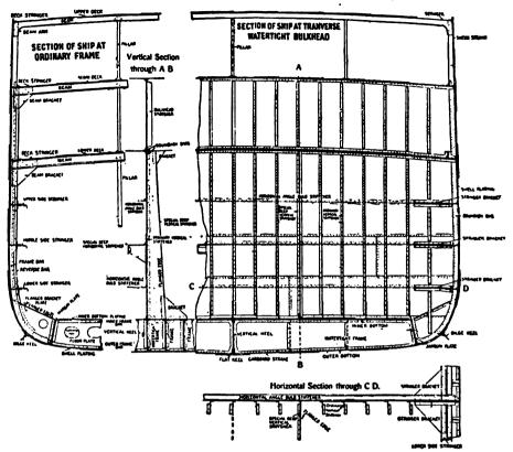
FIG. 113.-Details of Framing and Bulkheads.
