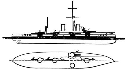
Fig. 63.—Arrangement of Guns and Armour. H.M.S. "Dreadnought."
