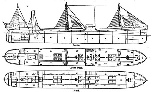
Fig. 12.—General Arrangement of a Modern Oil-Tank Steamer.
