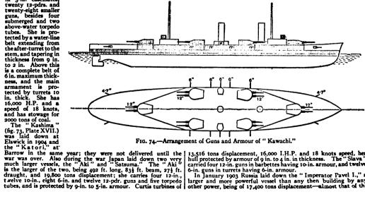
Fig. 74.—Arrangement of Guns and Armour of "Kawachi."
