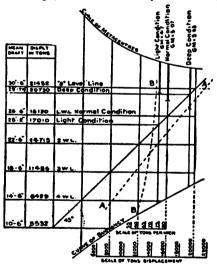
Fig. 3.-Metacentric Diagram of a Battleship.
