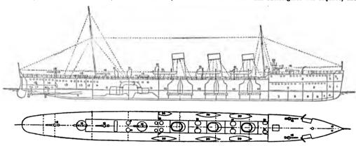
Fig. 118.-Torpedo-boat Destroyer "Swift."
