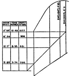
FIG. 5.-Metacentric Diagram of a Sailing Ship of "Symondite"
