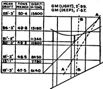
FIG. 4.-Metacentric Diagram of a Merchant Vessel.
