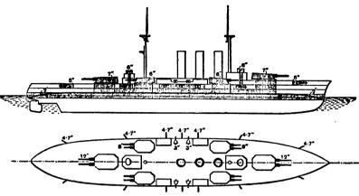
Fig. 106.—Arrangement of Guns and Armour, Japanese "Ibuki" and "Kurama."
