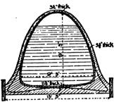
Fig. 28.—Reinforced Concrete Sewer. Section. inforcement per
