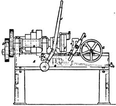
Fig. 3.-Bolt-Screwing Machine (John Stirk & Sons, Ltd., Halifax).
