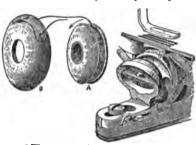
Fig. 6.—Rotary Hook, Bobbin, and Bobbin Case (Wheeler & Wilson Machine).
