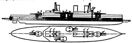
Fro. 96.—Arrangement of Guns and Armour of H.M.S. "Invincible."
