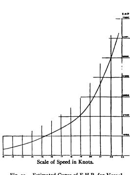
Fig. 39.—Estimated Curve of E.H.P. for Vessel  $320' \times 35\frac{1}{2}' \times 13' \times 2,135$  Tons.
