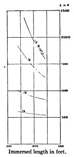
Fig. 45.—Curves of E. H. P. for 1,000-ton Ship. Group "A." Type 6. Block Coefficient .542.
