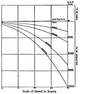
Fig. 38.—Curves of Surface Friction Correction.
