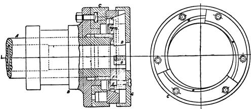
Fig. 4.—Opening Die-head for Screwing Machine.
