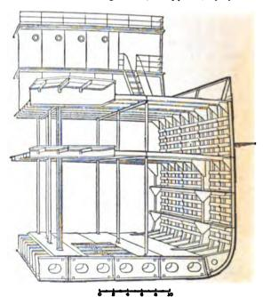
Fig. 111.—British Cargo Steamer; midship portion, in perspective.
