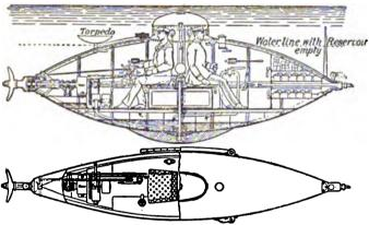
Fig. 127.—Section of Goubet Submarine Torpedo-boat.
